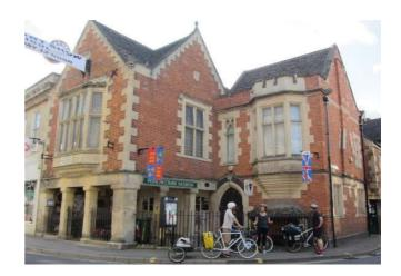
The appeal is for repairs to the two limestone pillars and the limestone lintel, which hold up the wing of the town hall which fronts on to Winchcombe High Street. As can be seen from these photographs, these pillars and lintel are structurally essential, which makes these repairs both vital and complex. This is further complicated by the narrowness of the pavement in front of the building.
